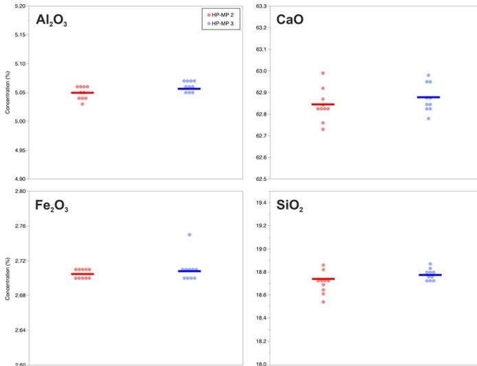
**Figure 2:** Graphical display of XRF analysis of concentration of Al<sub>2</sub>O<sub>3</sub>, CaO, Fe<sub>2</sub>O<sub>3</sub> and SiO<sub>2</sub> after sample preparation in the HP-MP 2 (red) and HP-MP 3 (blue).
