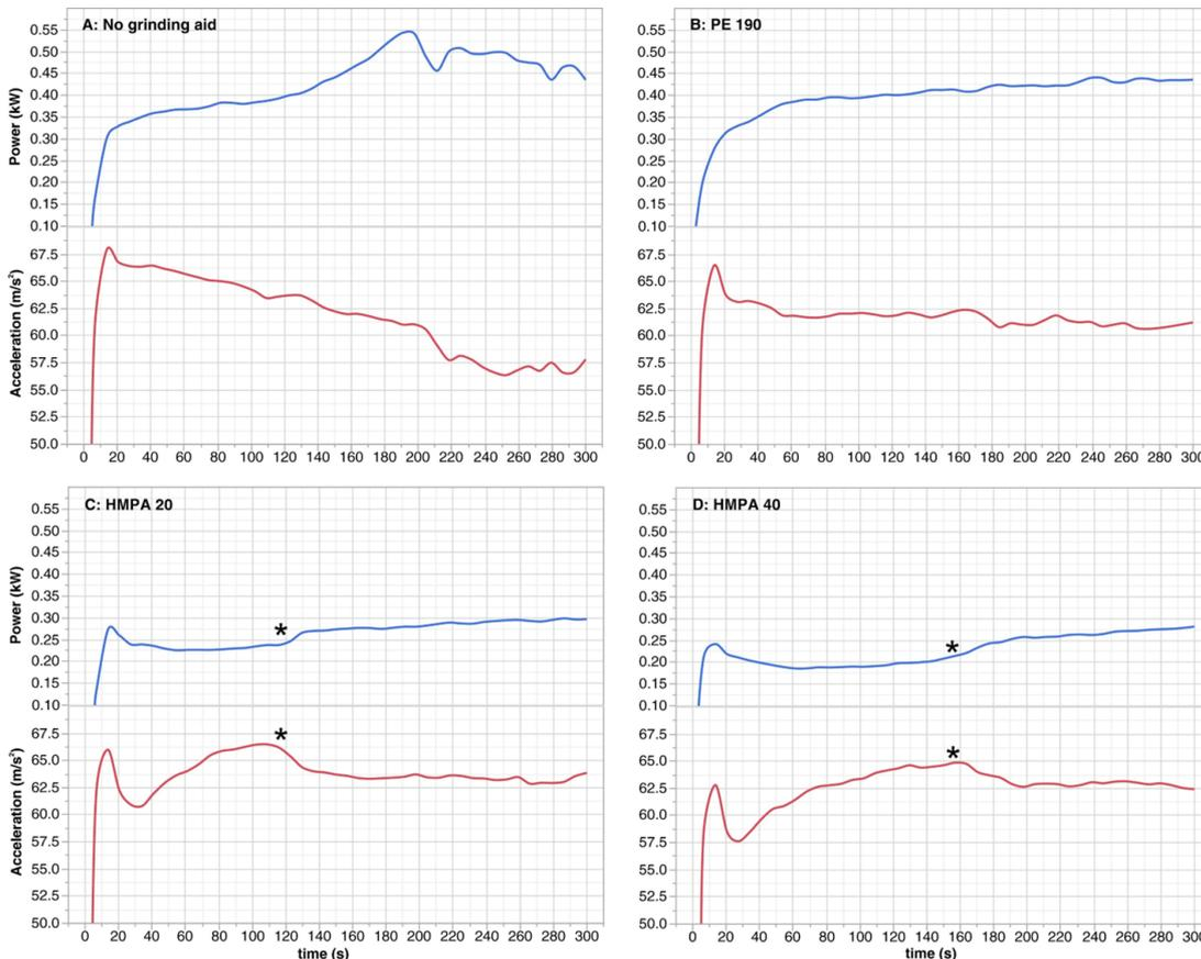
**Figure 2:** Display of the time course of grinding power and acceleration of the grinding vessel during the 300 s grinding trials.
