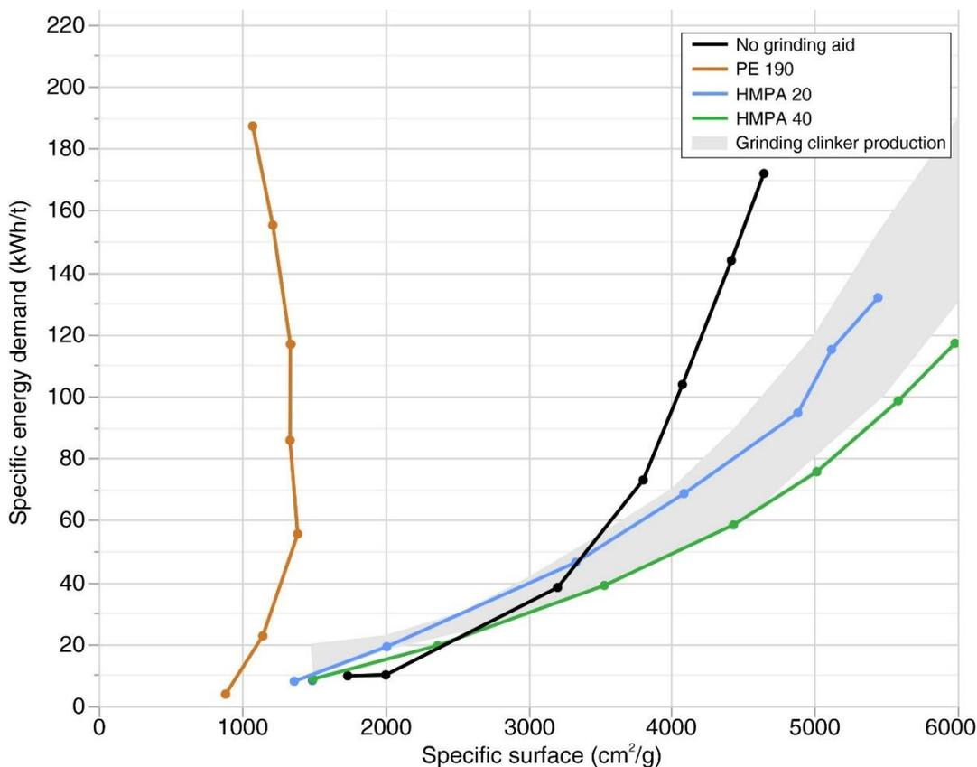
**Figure 1:** Graphical display of the specific energy demand for grinding of OPC clinker. To obtain the characteristic curves, the specific energy was plotted over the specific surface area measured at different times.
