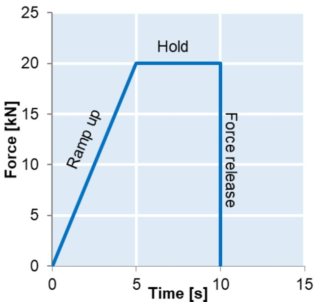
**Figure 2:** Sample preparation process. The final pressing force of 20 kN was ramped up for 5 s and released immediately after 5 s of force hold duration.
