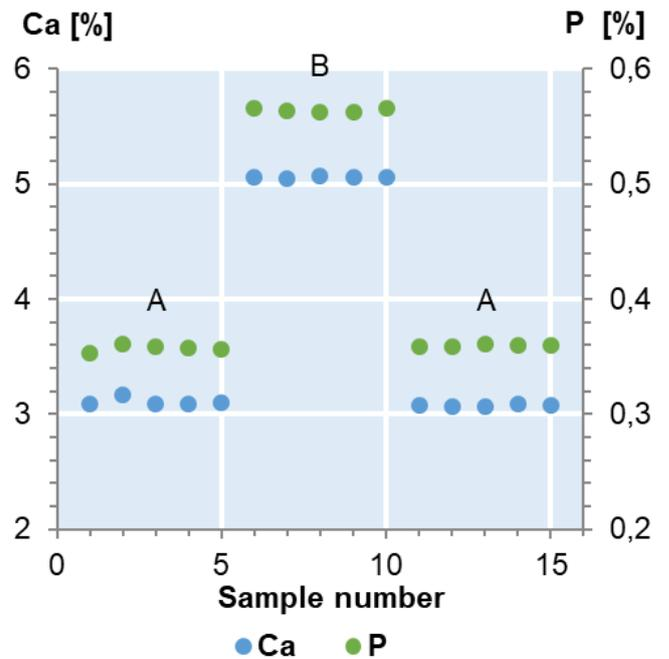
**Figure 3:** Results for Ca (blue) and P (green). Five samples of type B were prepared in between samples of type A. Automatic routine cleaning was used in between samples.
